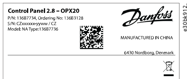
Figure 65: Example of a Control Panel Label
