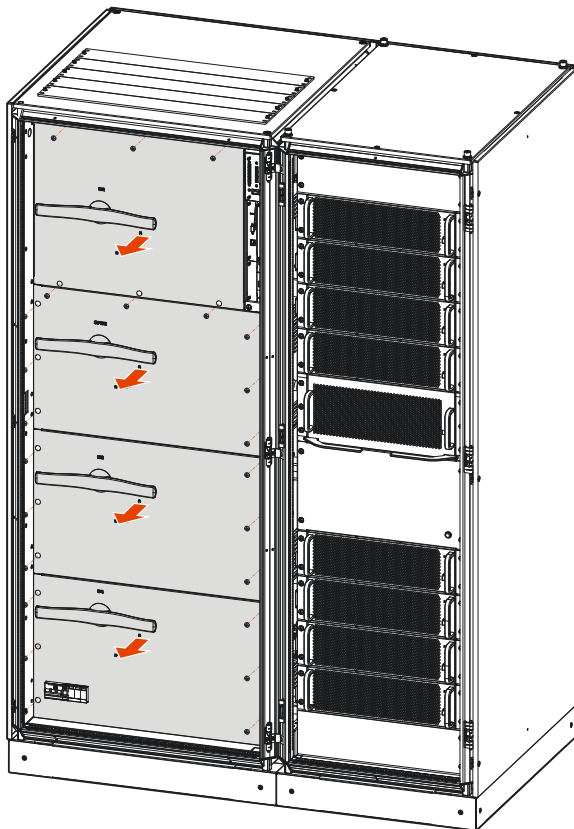
Figure3-26 Dismantle the wiring plates of distribution cabinet
