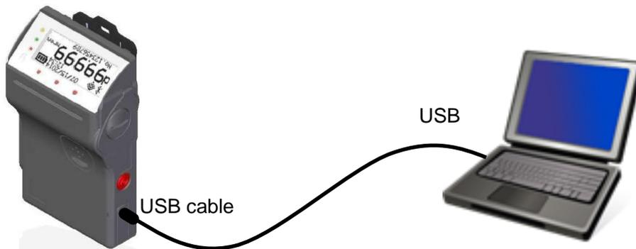
\* While connecting USB, IR device does not work.
