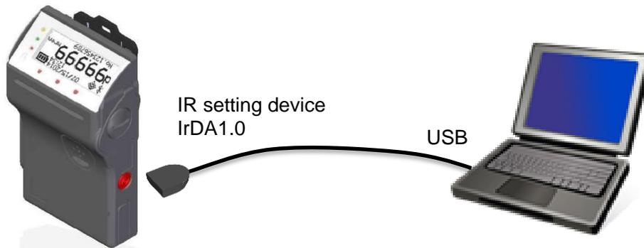
\* IR reception is located at lower left on the back of dosimeter.
