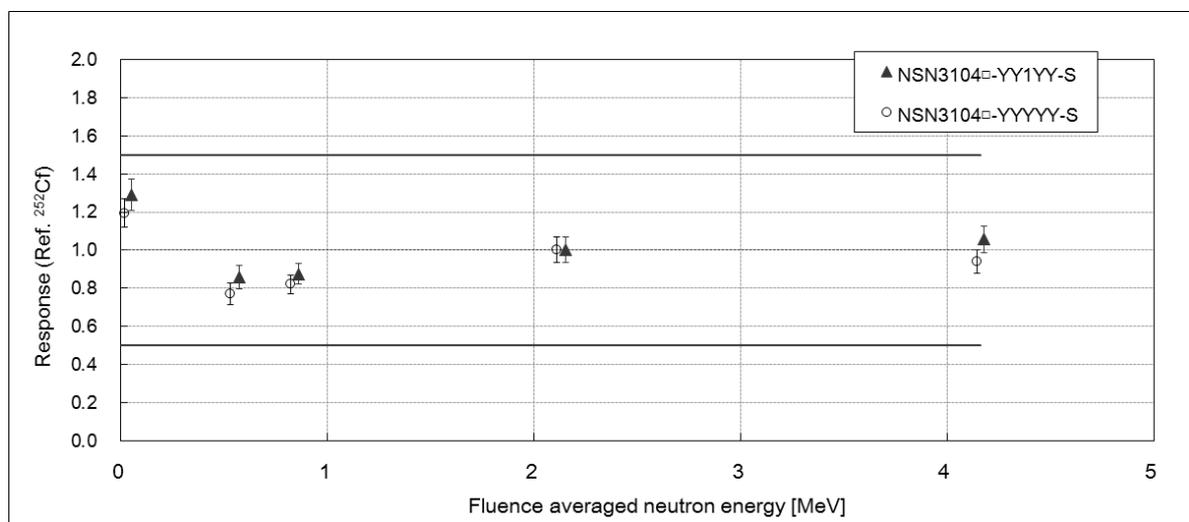
Figure 9-2-1 Energy characteristics for continuous energy neutrons
