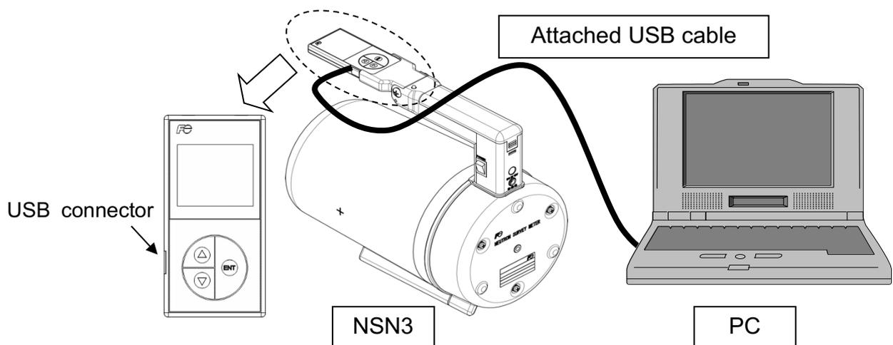
Figure 11-2 System configuration for the data transfer
