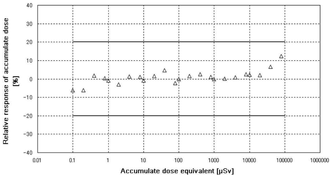
Figure 9-1-2 Relative intrinsic error of accumulate dose equivalent
