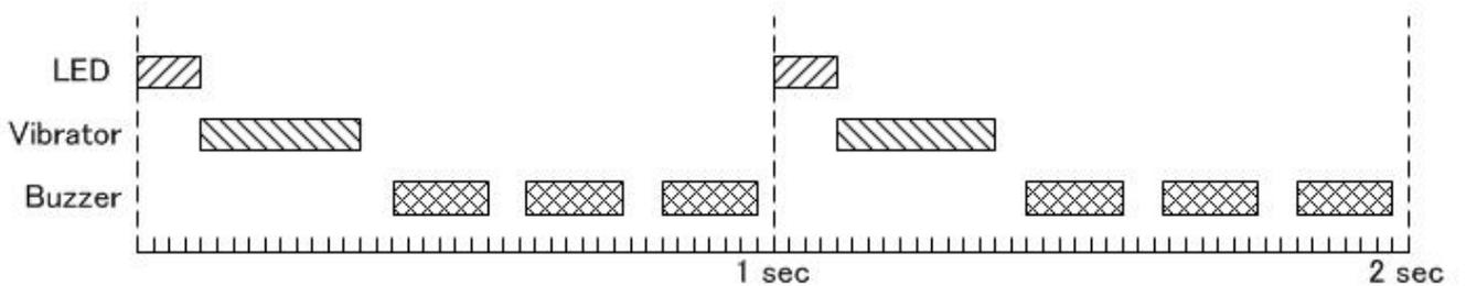
[Pattern No.4] ... When alarm is generated, the operating timing is showed below.
