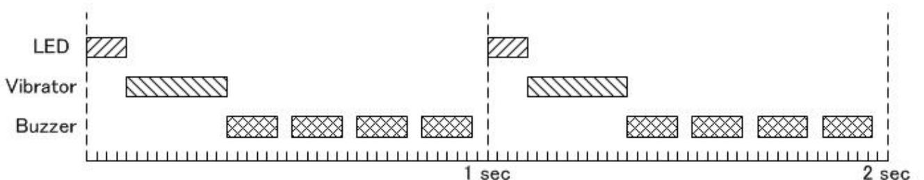
[Pattern No.5] ... When alarm is generated, the operating timing is showed below.
