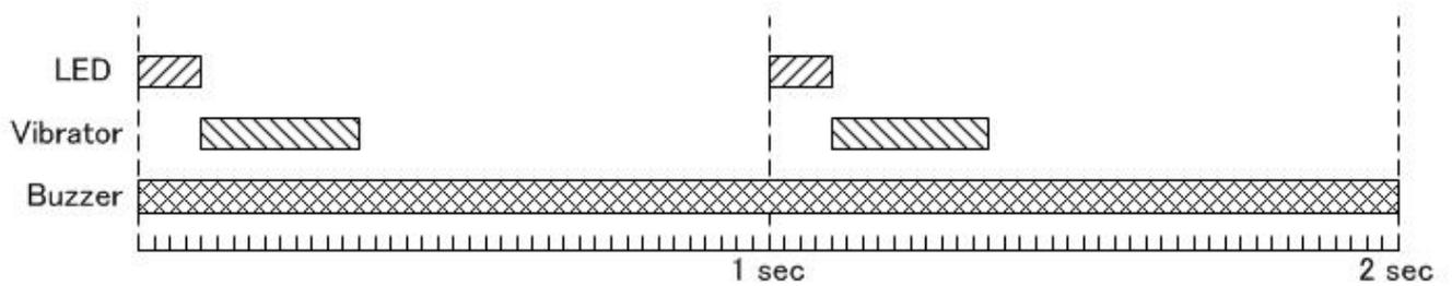
[Pattern No.6] ... When alarm is generated, the operating timing is showed below.
