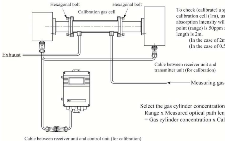
To check (calibrate) a span point by using the standard calibration cell (1m), use 100ppm gas cylinder. So, the absorption intensity will be same as that where the span point (range) is 50ppm and the measured optical path length is 2m.
