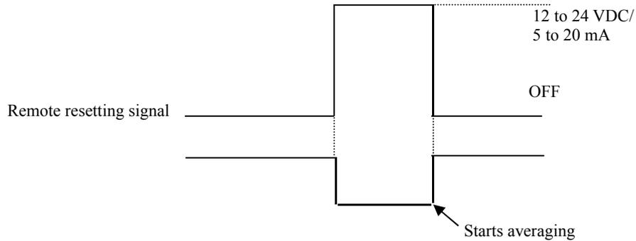
Reset is kept during short-circuit.
