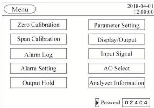
Enter "02404" to the Password. Select the digits by the key, and press the key or the key to move the cursor to "Password".
