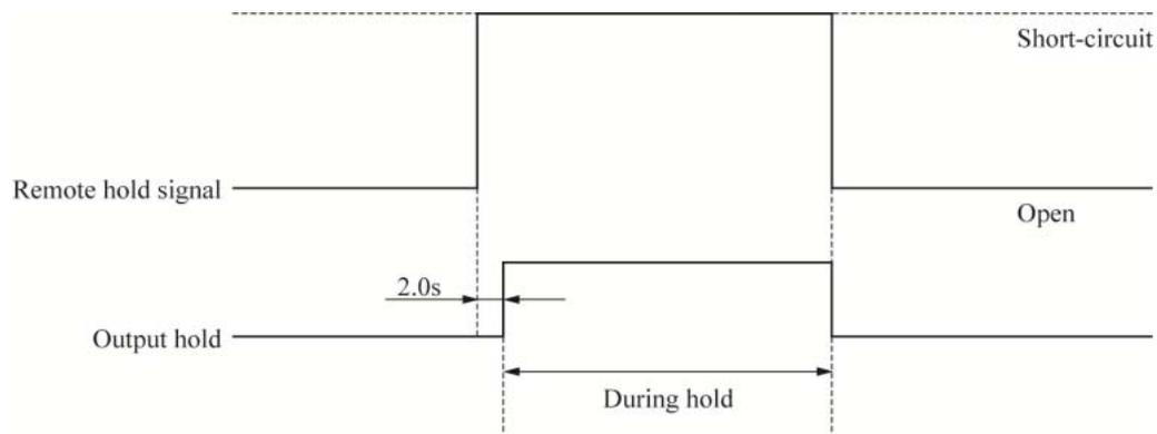
By applying a voltage (pulse width 2.0 seconds or more) to the remote hold input terminal, you can hold the analog output. The hold is cancelled when you stop applying the voltage.
