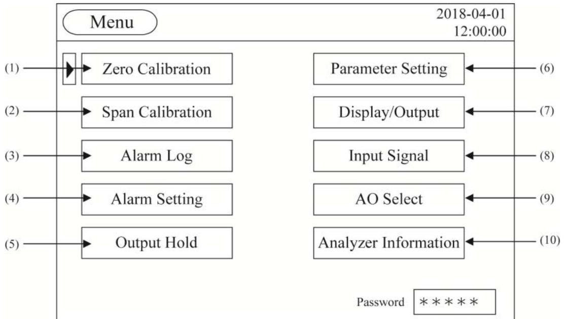
Press the **(MODE)** key while the “Measurement” screen is displayed, and the “Menu” screen appears. (It does not appear when pressing the **(MODE)** key while other screen is displayed. In that case, Press the **(ESC)** key to display the “Measurement” screen, and then press the **(MODE)** key.)
