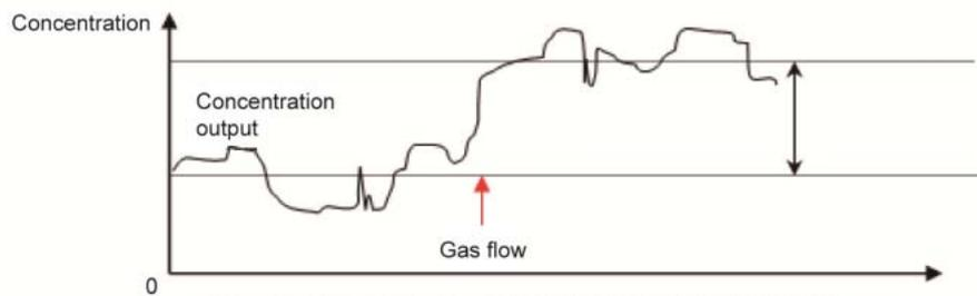
If gas concentration to be measured in the stack is not stabilized, it is difficult to measure the span point.
