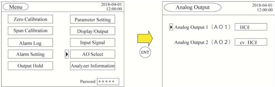
When the number of the components to be measured is one, “Component” or “No” can be selected. When there is O<sub>2</sub> conversion output, “O<sub>2</sub> Conversion” is also selectable.
