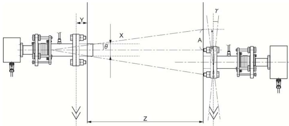
X: Flange inner diameter of receiver unit and transmitter unit
