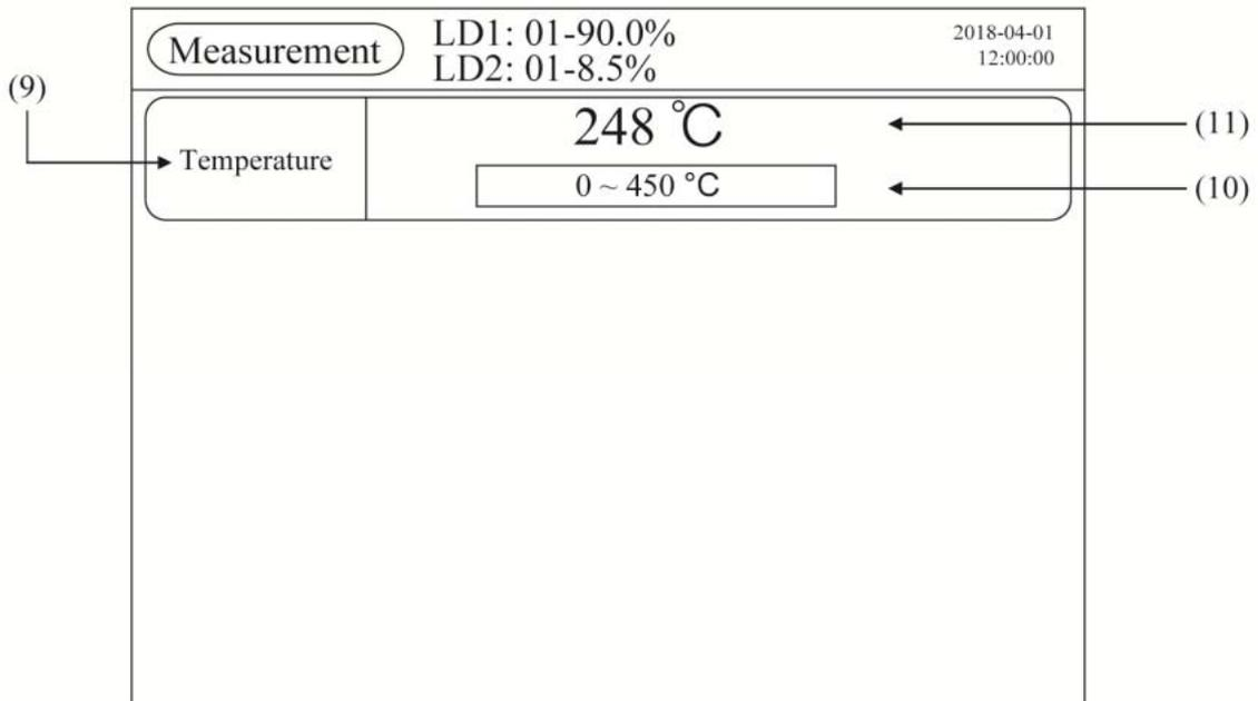
On the measurement screen, the display shows the components being measured, alarm, reference-O<sub>2</sub>-corrected concentration, and analog input. If there are more than four items to be displayed, use UP, DOWN or ENT to move up, down, or across the screen.
