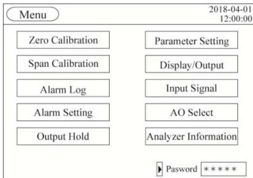
Point the cursor to "Password" in the bottom left of the "Menu" screen by the key or the key.
