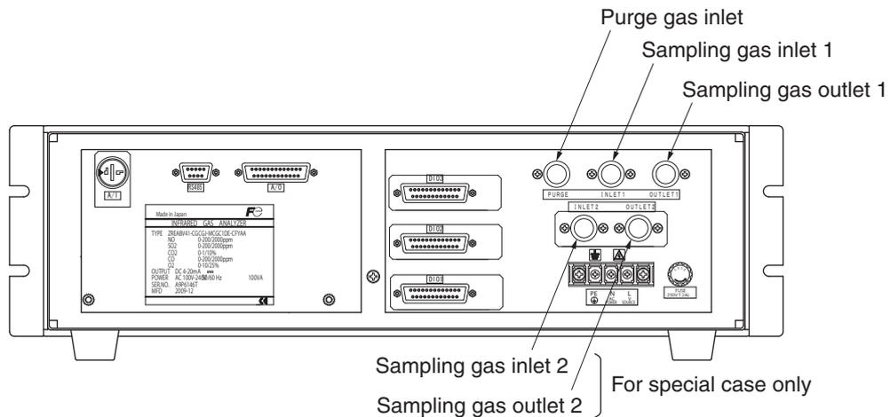
**Sampling gas inlet:** Attach the gas tube to introduce gas to be measured such as one that has completed dehumidification process and standard gases for zero and span calibration to this inlet.
