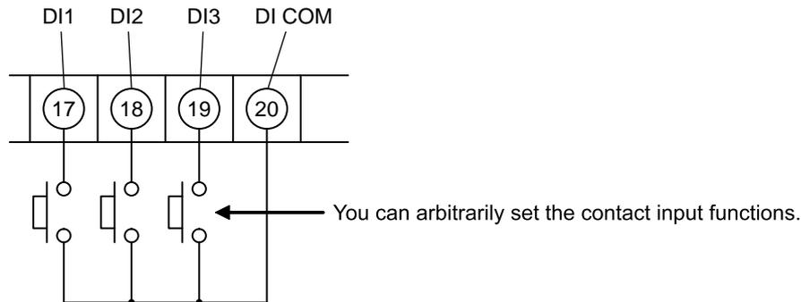
You can arbitrarily set the contact inputs (17), (18), (19) and (20) of the external terminal block (see “10.5.2 Contact input setting”).
