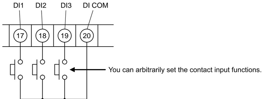
You can arbitrarily set the contact inputs (17) to (19) and (20) of the terminal block (see “10.5.2 Contact input setting”).
