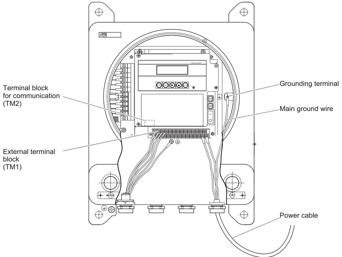
Note 1: Fix the exclusive cable (O<sub>2</sub> sensor input / O<sub>2</sub> sensor thermocouple input) with the cable gland so that its sheath is 10 mm or less.
