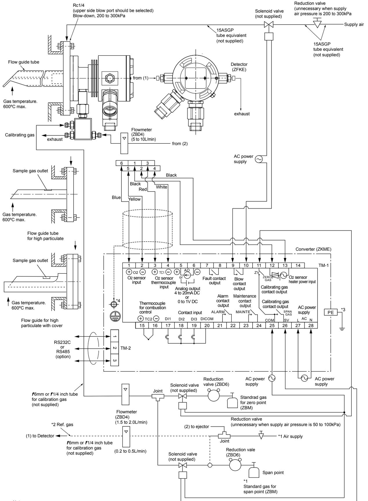
Note: \*1 Standard gas or instrumentation air can be used in place of span gas.
