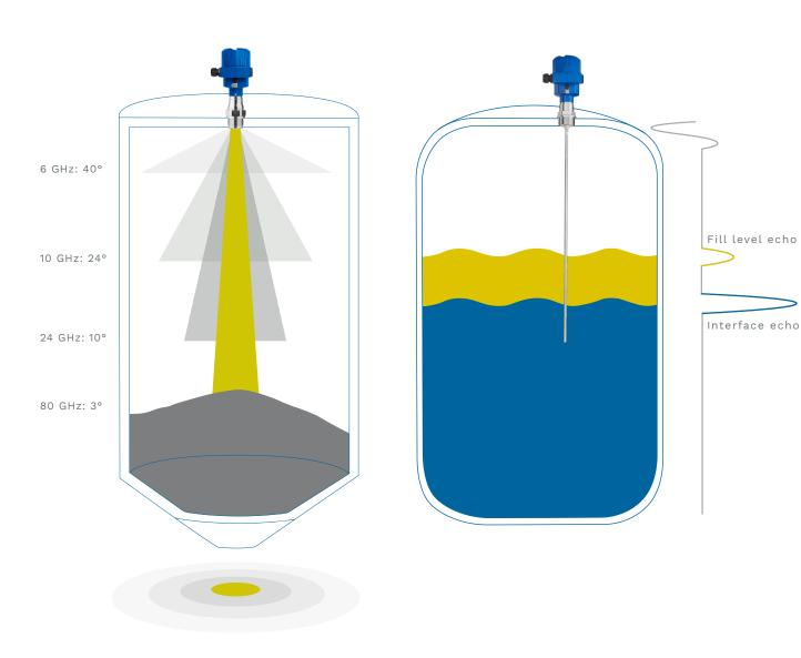
Bulk material measurement with bulk cone: The beam angle increases significantly as the frequency decreases – the 80 GHz technology offers the highest precision with just 3° Interface measurement of liquids with different DK values: The microwave pulse reflects off the upper layer (e.g., oil), penetrates it, and is reflected at the lower layer (e.g., water) back to the sensor.
