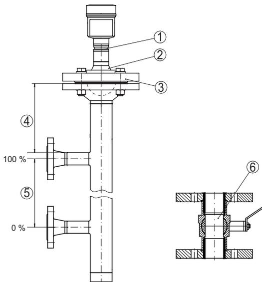
Fig. 23: Structure du tube bypass
