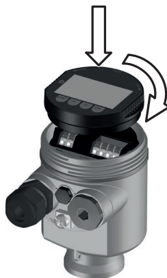
Fig. 43: Installing the display and adjustment module in the electronics compartment of the single chamber housing
