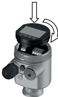
Fig. 41: Installing the display and adjustment module in the electronics compartment of the single chamber housing
