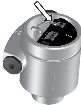
Fig. 28: Connection steps 5 and 6 - Single chamber housing
