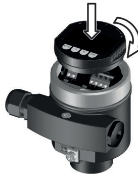
Fig. 32: Insertion of the display and adjustment module with single chamber housing
