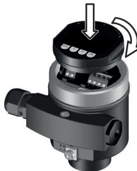
Fig. 28: Installing the display and adjustment module in the electronics compartment of the single chamber housing
