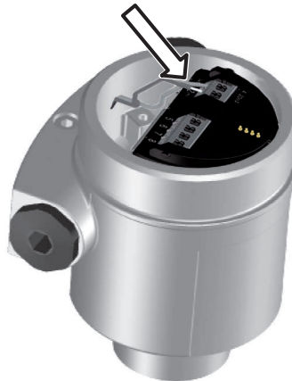
Fig. 21: Connection steps 5 and 6 - Single chamber housing
