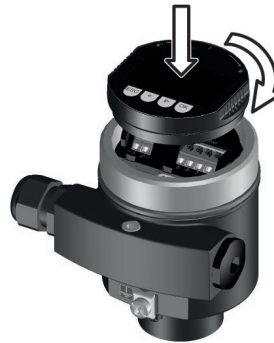
Fig. 23: Installing the display and adjustment module in the electronics compartment of the single chamber housing
