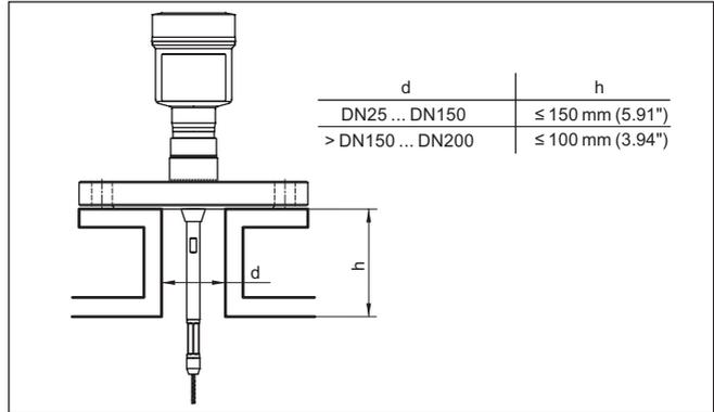
Fig. 4: Mounting socket
