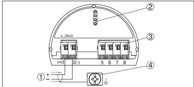
Fig. 7: Electronics and connection compartment - single chamber housing
