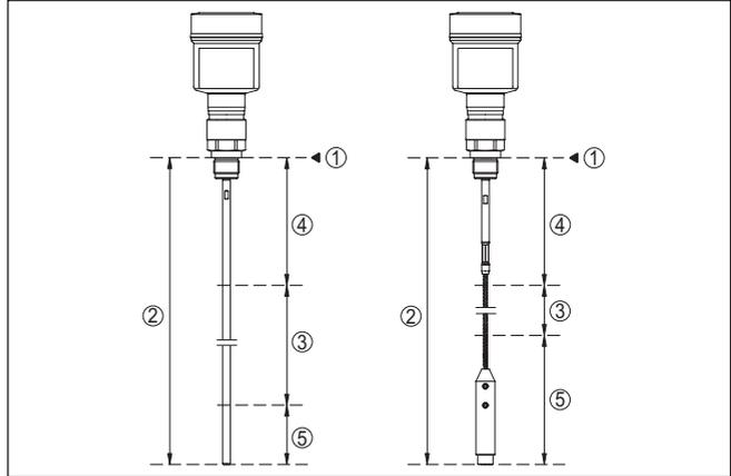
Fig. 11: Measuring ranges - NivoGuide 8100
