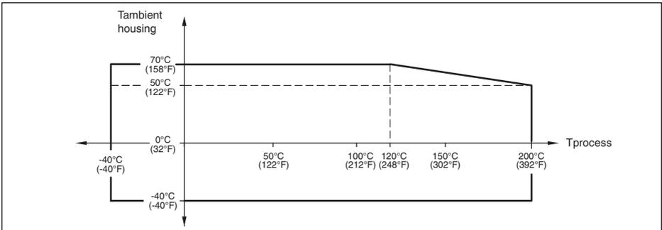
**Versions for process temperatures up to +250 °C with metal housing**
