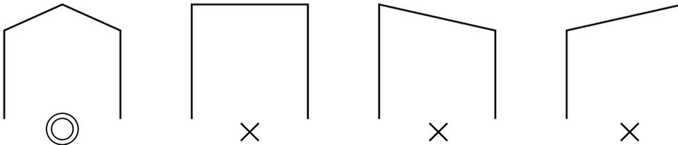
Insert the paper straight to the paper insertion section.
