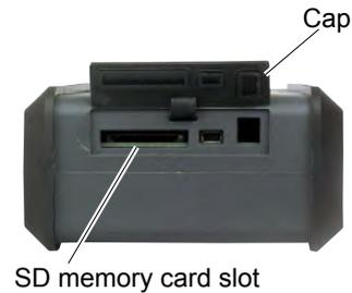
Step 2) Insert a memory card into the memory card slot in the main unit bottom face in the direction shown on the right. Card push-in system is adopted for card mounting. Positively push in the memory card to the lock-up position.
