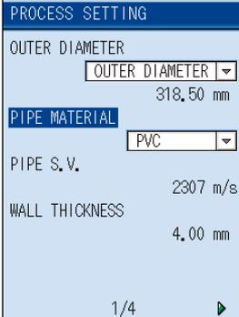
The screenshot shows the 'PROCESS SETTING' screen. The 'OUTER DIAMETER' is set to 318.50 mm. The 'PIPE MATERIAL' dropdown is set to 'PVC'. The 'PIPE S.V.' is set to 2307 m/s. The 'WALL THICKNESS' is set to 4.00 mm. A page indicator '1/4' is visible at the bottom right.
