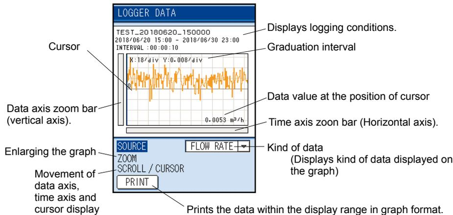
Logging data for up to four screens from the start of logging is displayed. The maximum number of data is 816 data (204 data per screen).
