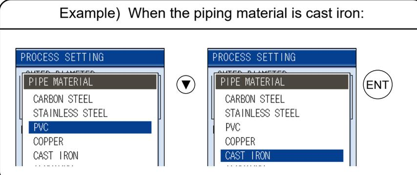
The diagram illustrates the process of selecting 'CAST IRON' as the piping material. It shows two sequential screenshots of the 'PIPE MATERIAL' selection screen. In the first screenshot, 'PVC' is highlighted, and a down arrow key is shown next to it. In the second screenshot, 'CAST IRON' is highlighted, and an 'ENT' key icon is shown next to it.
