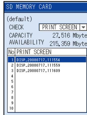
(2) Press the **ENT** key on the SD MEMORY CARD screen and the CHECK screen appears.
