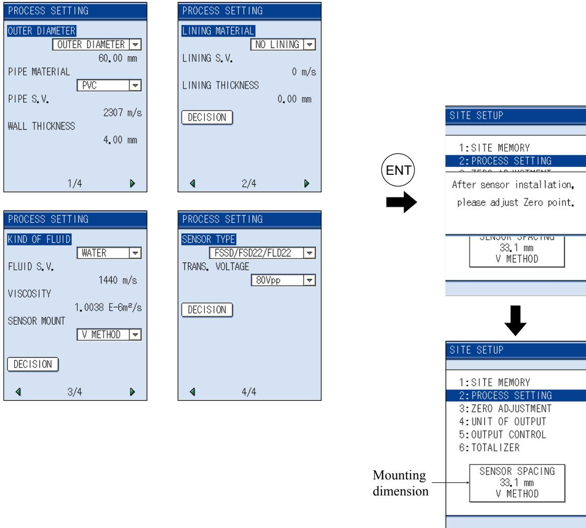
Install the sensor according to chapter 8. MOUNTING OF DETECTOR and the mounting dimension is as displayed on the last line.
