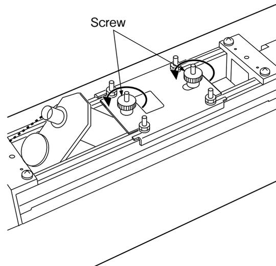
**(5) Connect the detector and the converter unit**
