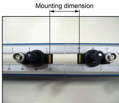
(4) Apply the acoustic coupler on the transmission surface of the sensor unit.
