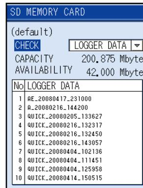
(3) Move the cursor to the data items to be checked (LOGGER DATA, PRINT SCREEN and FLOW PROFILE) by the **▲** or **▼** key and press the **ENT** key.
