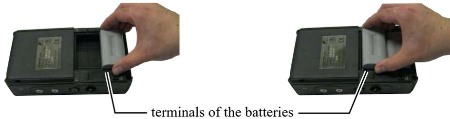
(3) Two battery packs are inserted in place.
