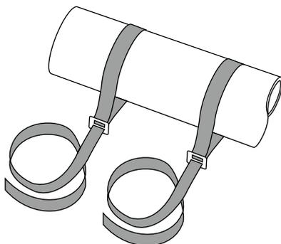
Adjusts the length of the wire rope according to the piping size, fixes the wire on the pipe.
