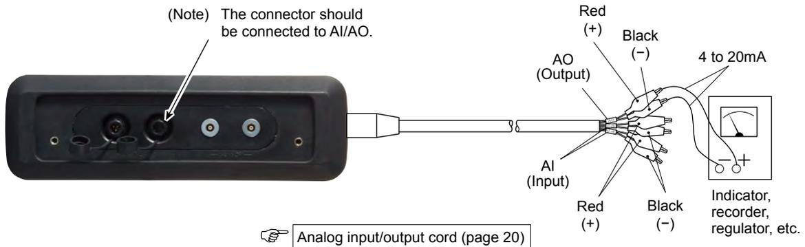
Analog output: 4 to 20mA DC 1 point “Load resistance under 600Ω”
