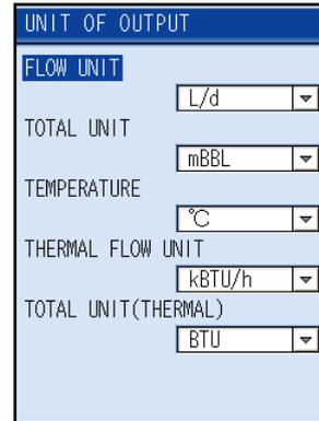
(3) Press the ENT key to open the unit selection screen. Select the unit by the ▲ or ▼ key and then press the ENT key.
