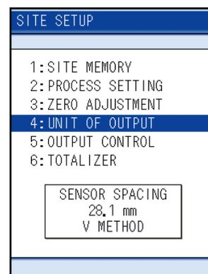
(2) Press the ▲ or ▼ key and move the cursor to the output item of which unit to be changed.
