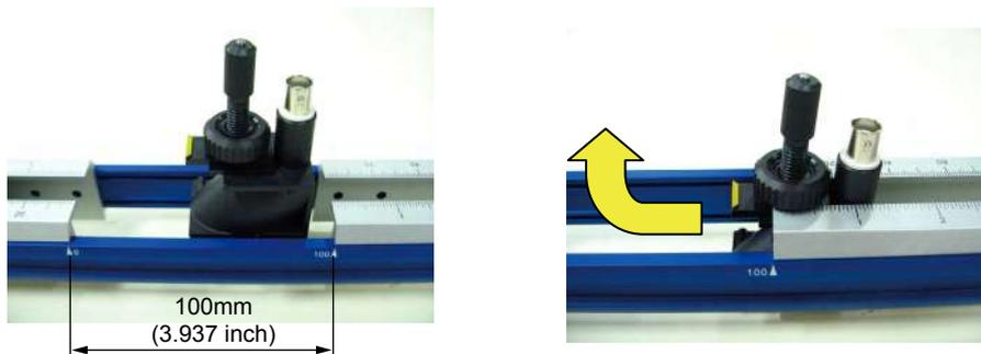
(3) Loosen the lock nut and adjust the mounting dimension of the sensor unit.
