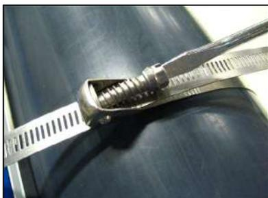
3-4) Make sure the tension of the belt and make an adjustment.
