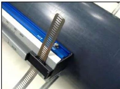
3-2) Put the belt through the fixing clamp.
