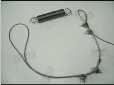
4-2) Put the wire through the hole of rail end and wrap it around the pipe and hook it with mounting spring to fix. Mounting spring length is approx. 180mm.
