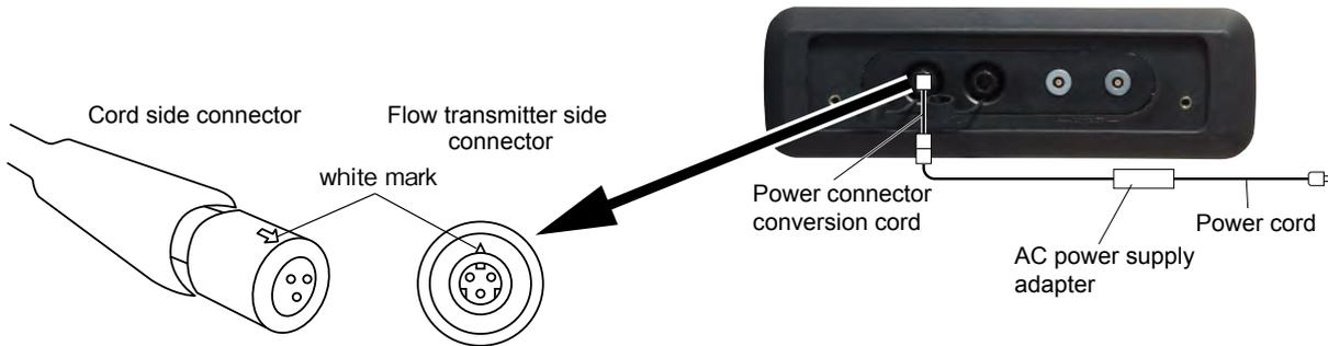
(2) Insert the power cord plug to the AC power socket (100–240 V AC, 50/60 Hz).
