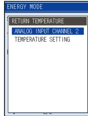
Note1) To set the feed/return temperature to the fixed temperature (TEMPERATURE SETTING), make settings for feed/return temperature on the ANALOG INPUT CHANNEL1 and ANALOG INPUT CHANNEL2 screen.
