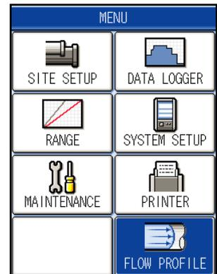
(3) Press the **ENT** key twice, flow velocity profile screen will display.
