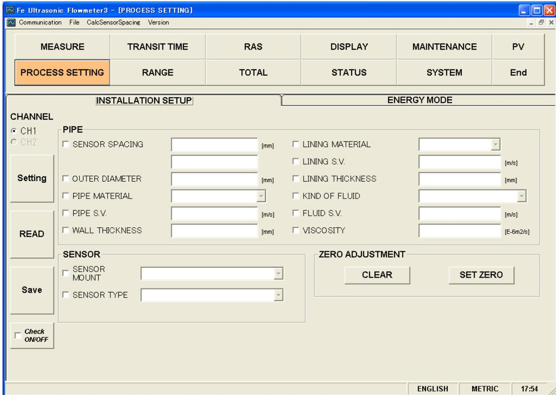
Fig. 9-16 < Installation setting screen >
