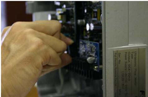
Pull out the card relay from socket.
