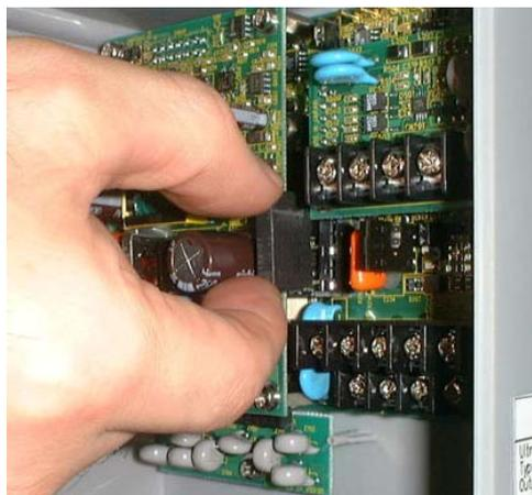
Pull out the card relay from socket.
