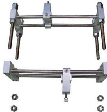
Fig. 5-4 Sensor mounting bracket separated
