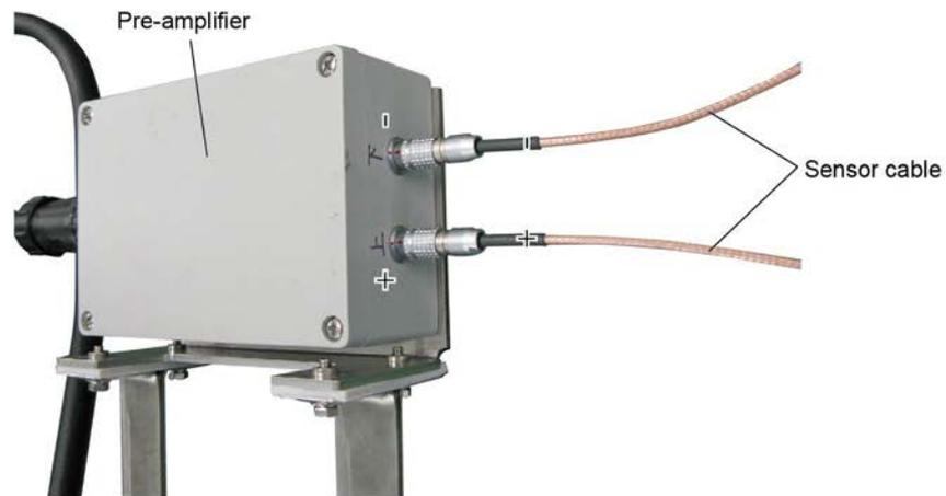
Insert the dedicated signal cable all the way in, and then tighten the screw.
