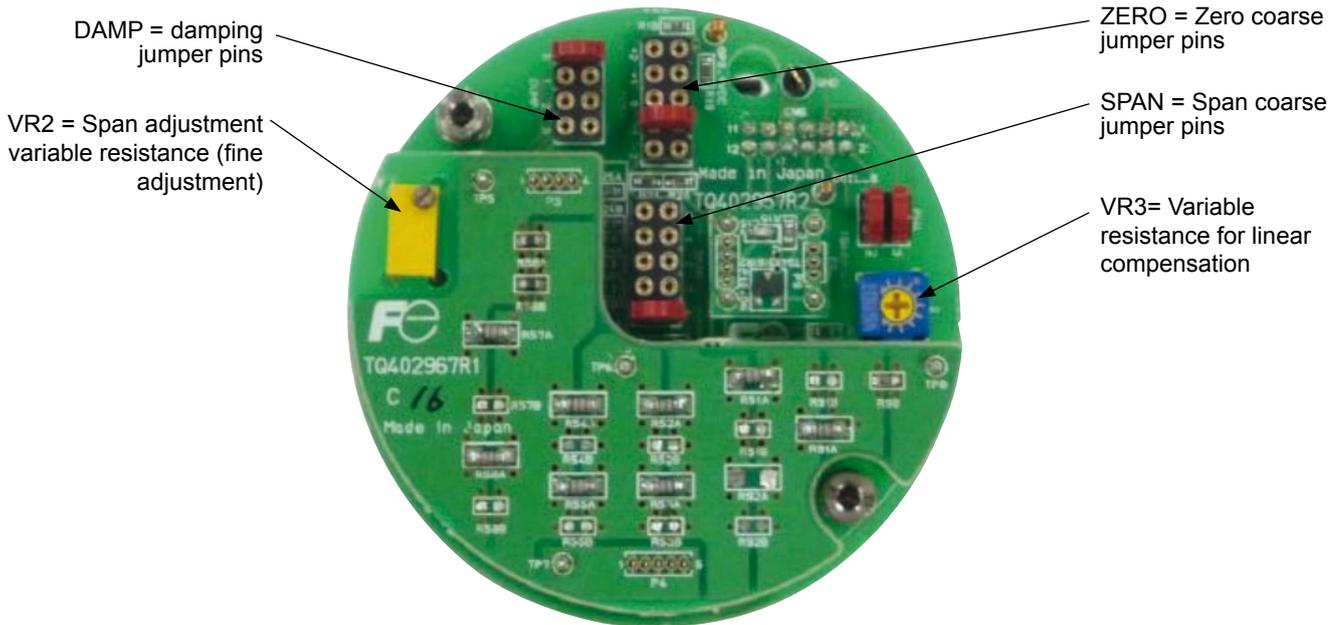
Top view of Analog Transmitter Amplifier
