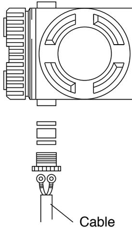
In case of SOURIAU or SAIB socket, a female quick connector enables to perform the wiring.
