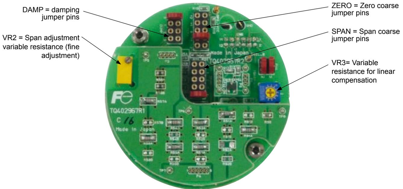
Top view of Analog Transmitter Amplifier
