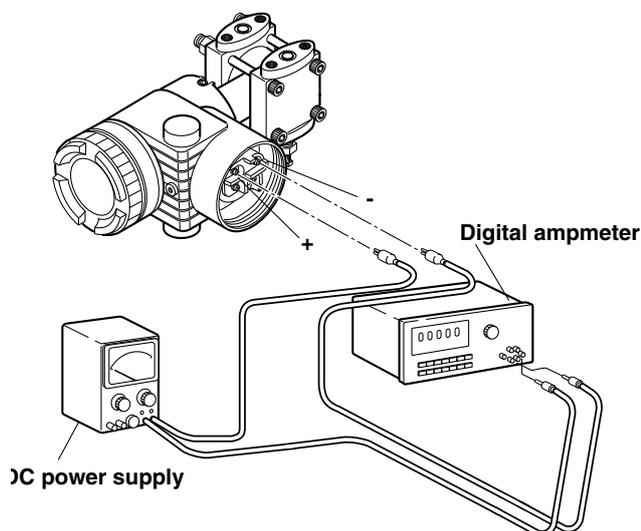
(2) Perform the calibration of either zero or span as described in the section 6.1.1 and 6.1.2
