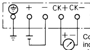
Connection of local analog indicator, or remote indicator of current 4/20mA loop test milliampmeter. (max impedance = 12Ω)
