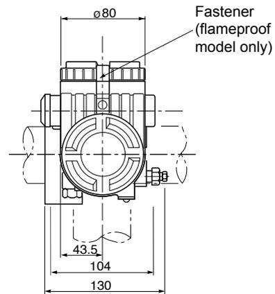
"Side vent/drain" configuration (11th digit : D & F)
