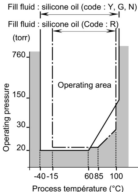
Fig.1 Relation between the temperature of process in contact with cell's diaphragms and operating pressure.
