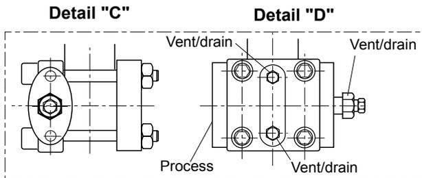
With this configuration, vent/drain function on the **external side** of the process flanges is achieved by way of vent screws directly attached to the flange (sealing is of metal to metal type). There is no more conventional screwed vent seat screwed in the flange and sealed with "PMCU Loctite" type compound.
