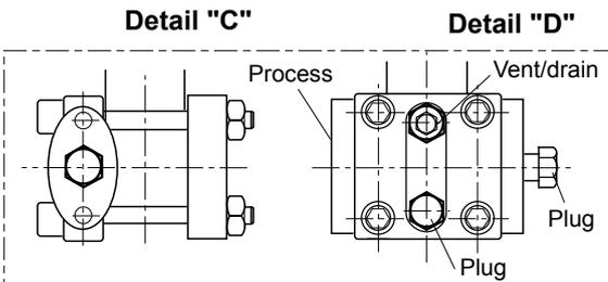
"Universal vent/drain, direct mounting" configuration (11th digit : G & H) (recommended for UTO stock)
