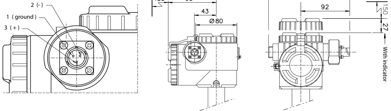
**Conduit connection SAIB connector (4th digit = code 8)**
