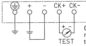
Connection of local analog indicator, or remote indicator of current 4/20mA loop test milliammeter.
