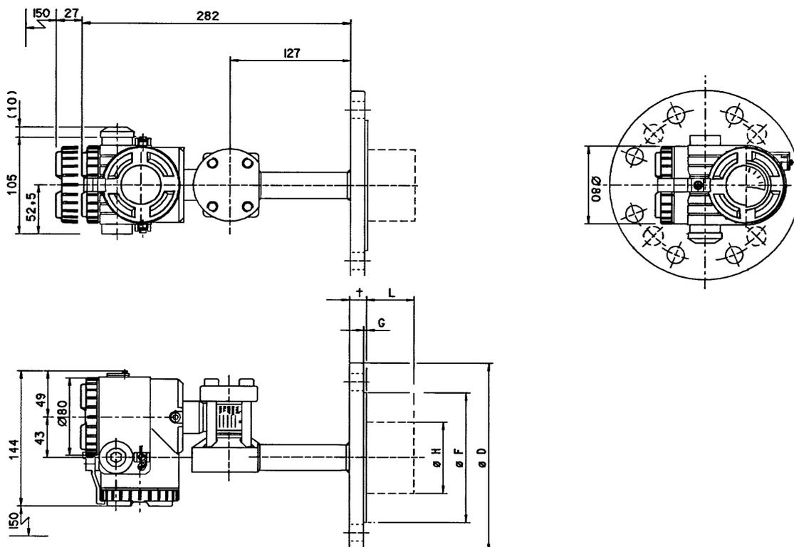
**Outline dimensions for capillary mounted diaphragm seal(s) on a differential pressure transmitter** (units : mm)
