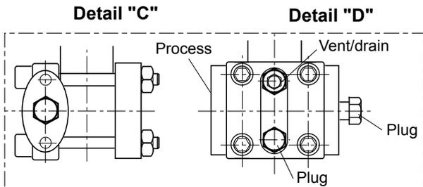
**"Universal vent/drain, direct mounting" configuration (11th digit : G & H) (recommended for UTO stock)**
