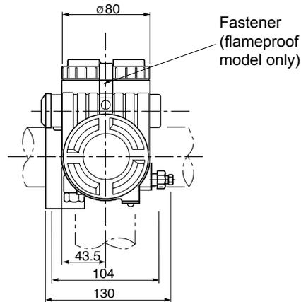
**"Side vent/drain" configuration (11th digit : D & F)**
