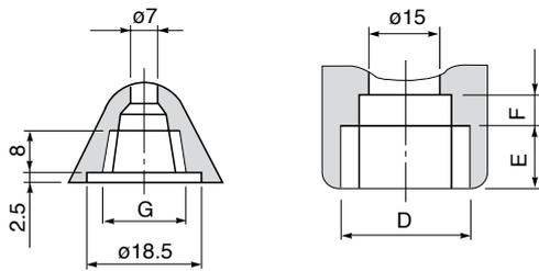
Detail "A" Process connection      Detail "B" Conduit connection
