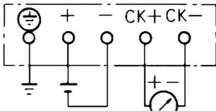
Connection of local analog indicator, or remote indicator of current 4/20mA loop test milliammeter. (max impedance = 12Ω)
