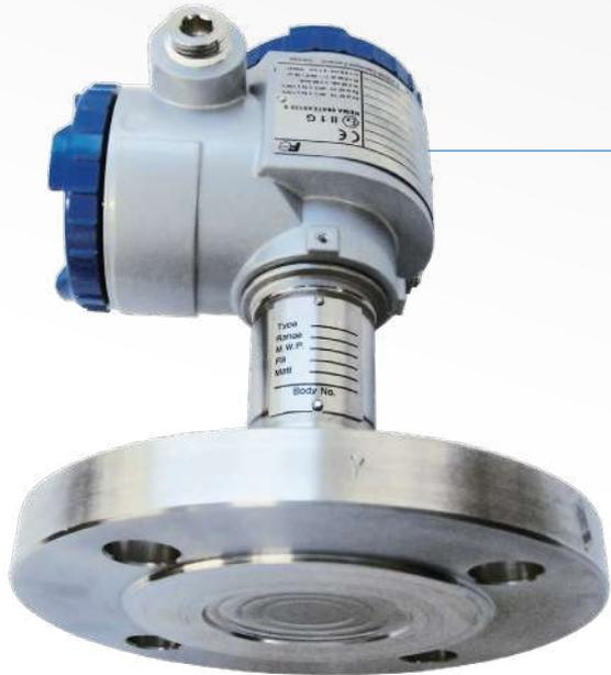
Remote seal with ceramic coating to protect the diaphragm against abrasion, often used in paper-making, oil industry, waste water treatment, powder transport, etc.
